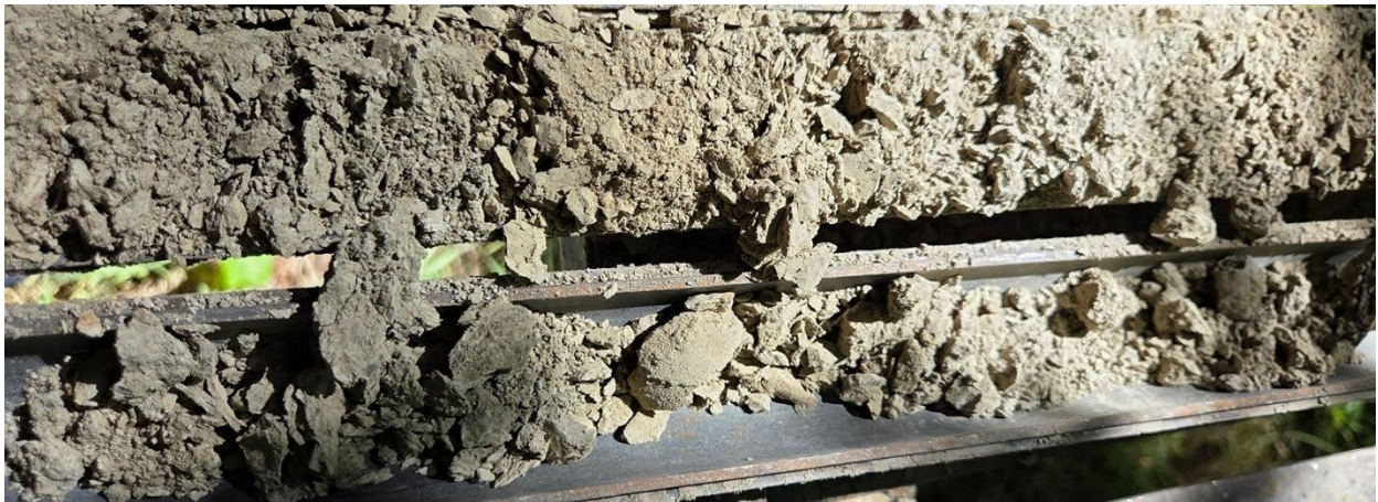
Plate 4 – Pre-Olympia, Non-glacial Fine Grained: Hard, sandy SILT (Qponf) | PG-1-25, S-4 @ 7½ – 9 feet.
